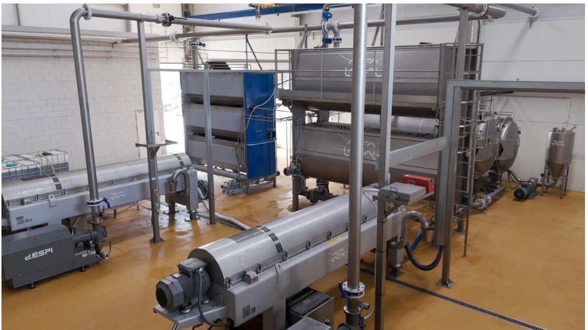
2. Alfa Laval's Foodec Sigma decanters at Coselva increase the extraction of premium extra virgin olive oil
