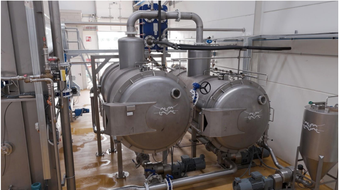
1. Alfa Laval's Olive Oil Booster at Coselva improves polyphenol content by up to 20%
