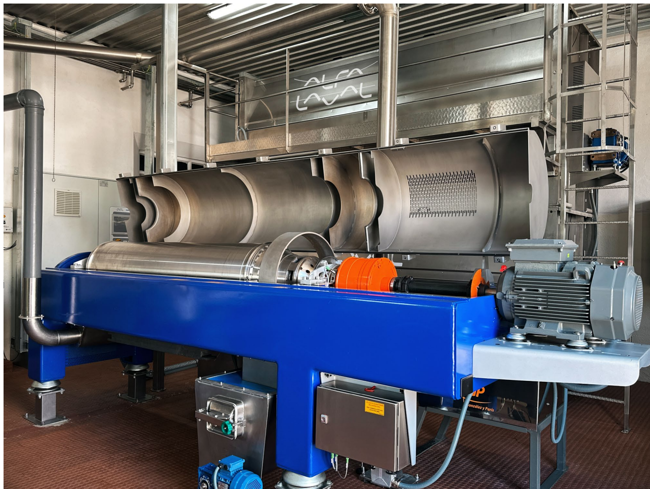
Alfa Laval's Foodec Sigma decenter, now operating at the Caminhos Do Futuro olive oil mill, represents a breakthrough in olive oil extraction
